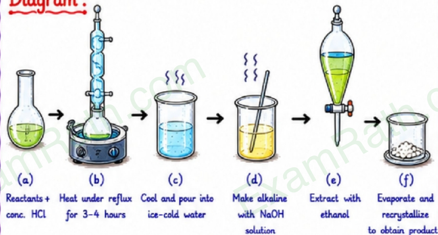
Figure 16 : Synthesis of Propranolol
